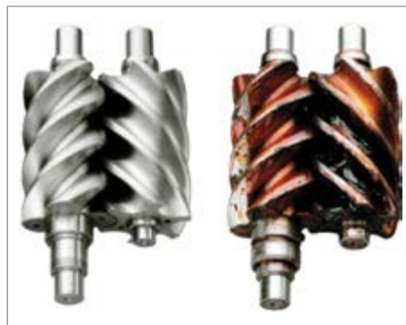
The Compressed Air Purity Guide notes, depending on the type of air compressor and compression temperatures, some air compressor lubricants can create varnish. (Photo courtesy of Hitachi Global Air Power US)
